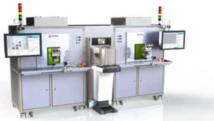
**Mikromotor Löten / Micro motor soldering**
